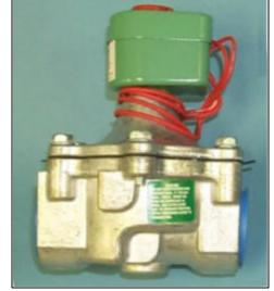
C with modifications and options. These are direct acting valves and have relatively quick response times. For the 1/4"-1/2" valves we have a response time number of between 10-20 msec. Special elastomers for chemically specific applications.
