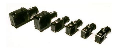
These six mechanical high vacuum pumps are the newest addition to the HYVAC line. They incorporate two stage design, with the basic oil sealed rotary vane principle. They are excellent general purpose or roughing pumps capable of vacuum pressures to 5 x 10<sup>-4</sup> Torr or .5 micron with fast recovery times. Since they are direct drive pumps, they offer high volumetric efficiency with ease of portability.
